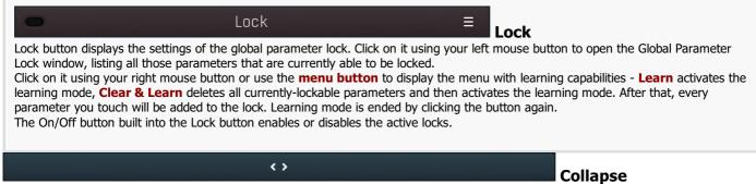
Collapse button minimizes or enlarges the panel to release space for other editors.
