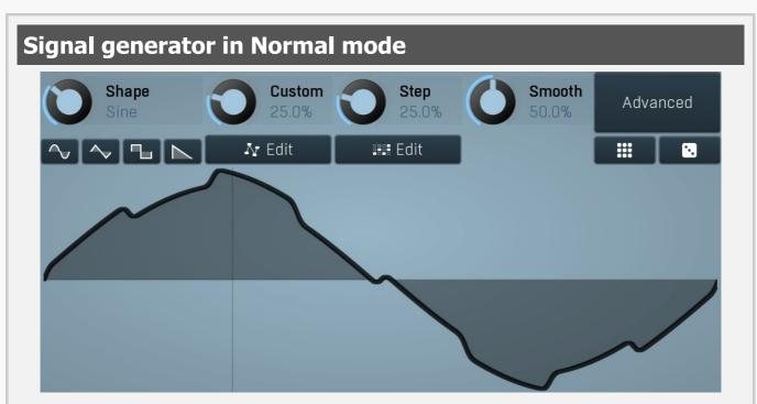
Signal generator in Normal mode works by generating the oscillator shape using a combination of several curves - a predefined set of standard curves, custom shape, step sequencer and custom sample. It also post-processes the shape using several filters including smoothing to custom transformations. This is especially useful when using the oscillator as an LFO (low-frequency-oscillator), where the harmonic contents does not really matter, but the shape does.
