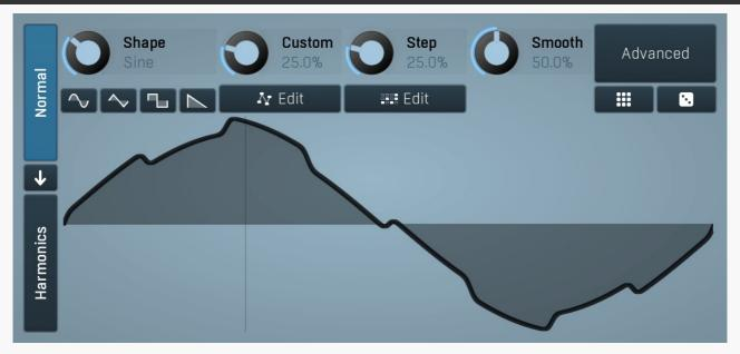
Signal graph defines the low frequency oscillator shape. Signal-generator is an incredibly versatile generator of low & high frequency signals. It offers 2 distinct modes - Normal and Harmonics.
