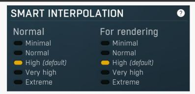
Smart interpolation panel controls the depth of the smart interpolation algorithm, which controls the parameters in order to provide maximum audio quality and lower the chance of zipper noise. Smart interpolation is engaged whenever you change any parameter via the GUI, modulators, multiparameters, MIDI or automation.
