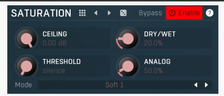
Saturation panel contains parameters of the master effect that is processed after the individual bands are processed and the signal is mixed back together.
