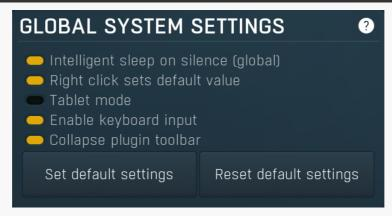
Global system settings panel contains settings which are applied to all plugins on this computer.
