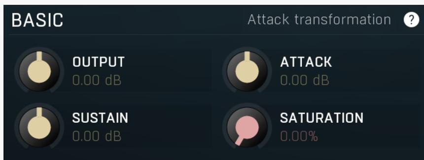
Basic panel contains the most important transient processor parameters.
