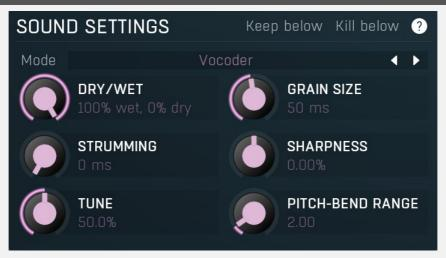
Sound settings panel contains properties of the algorithms used for pitch shifting and harmonization. They affect CPU consumption and sound quality.
