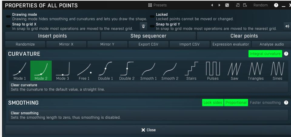
Envelope graph menu provides additional features which are used to edit the graph. Open the menu using right mouse button in the graph. Please note that if you select some points in the graph, or click on a point for example, the menu will be different and will cover only those features related to the selected set of points.
