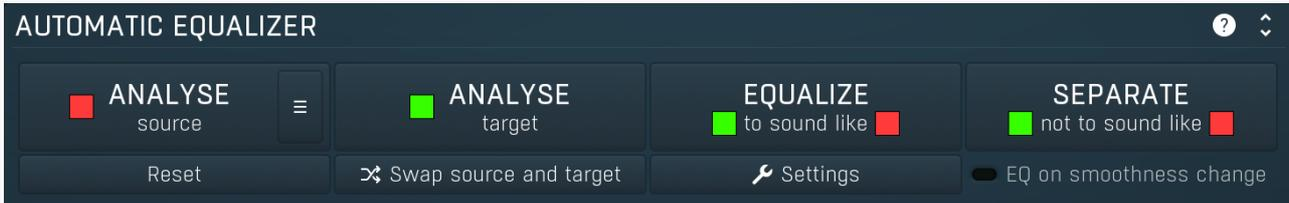
Automatic equalizer panel contains long-term analysis and automatic equalization functions.
