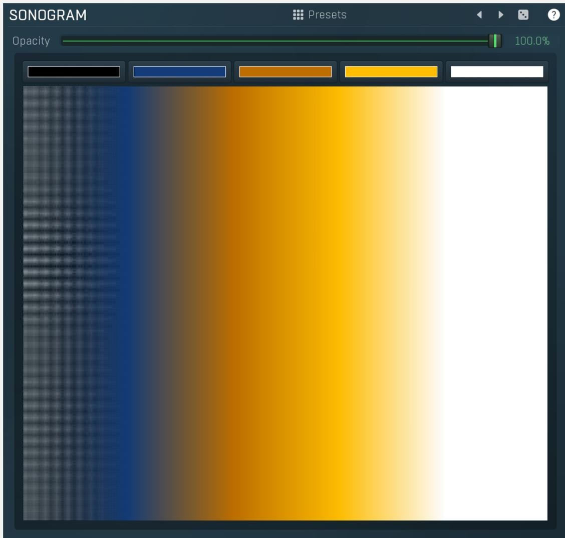
Sonogram panel contains visual settings of the sonogram, mainly the sonogram colors. A sonogram uses a set of colors. When the particular frequency's level is at the minimum, the first color is used. When it is at the maximum, the last color is used. Otherwise it interpolates the colors in-between.
