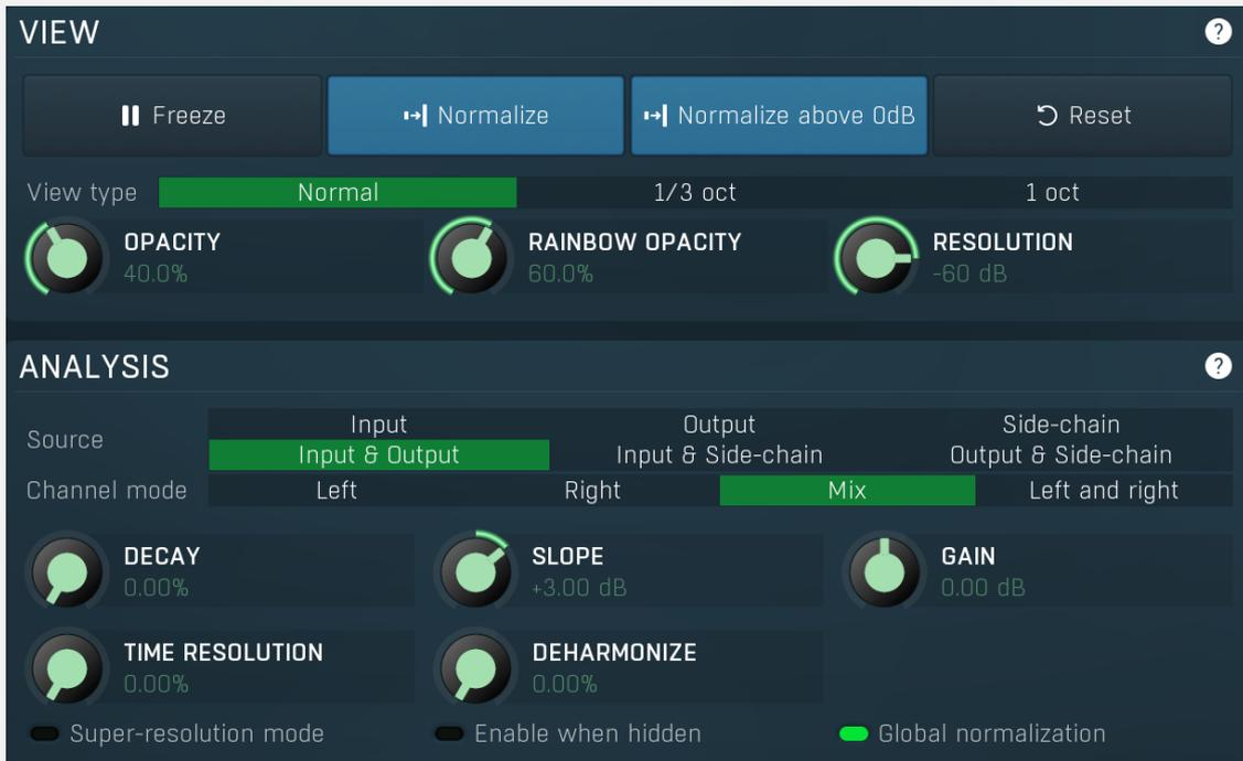
Main settings panel contains the most useful settings controlling the analyzer behaviour and view.
