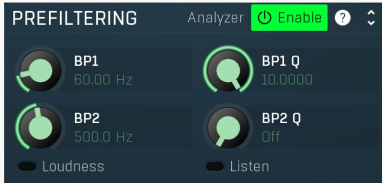
Prefiltering panel contains some filtering parameters that let you preprocess the detection signal. There are mainly 2 parallel band-pass filters, which let you specifically target 2 resonant frequencies in the signal and may come handy if you for example process a signal with lots of leakage, e.g. a hi-hat microphone which has recorded lots of leakage from the snare drum.
