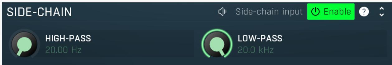
Side-chain panel lets you do additional filtering of the level detector input. Please note that its name does not mean it is related to the processor's secondary input (if it has one). Its main purpose is to filter the signal fed to the level detector. This is useful when, for example, you want to remove high volume peaks of a particular frequency.
