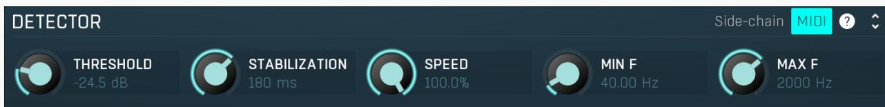
Detector panel contains advanced settings for the pitch detector that the plugin uses. Use the parameters to adjust it to your audio material.
