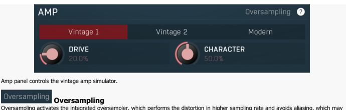
Oversampling activates the integrated oversampler, which performs the distortion in higher sampling rate and avoids aliasing, which may be especially noticeable for higher drive values. However note that this increases the CPU requirements extensively.
